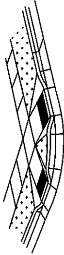
3-D View Type A-1 Sidewalk Ramp
