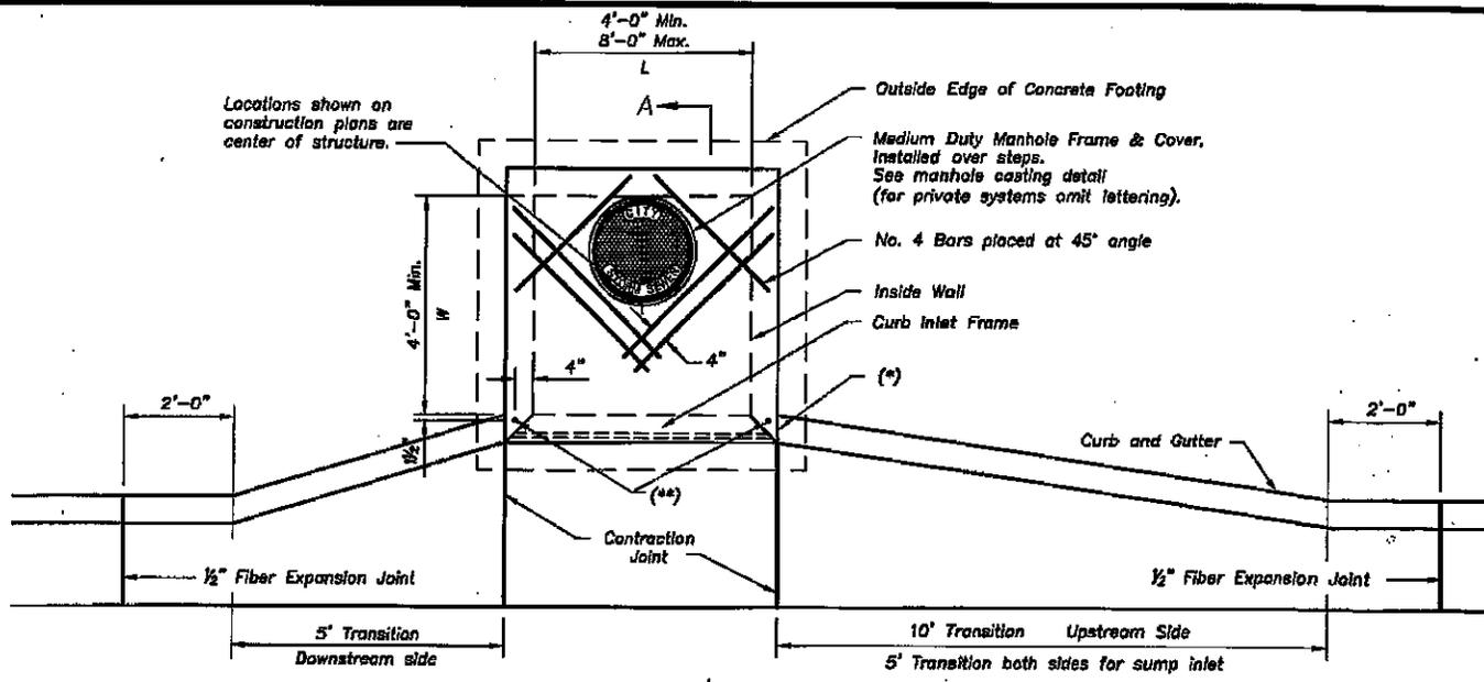
(\*) - Curb & Gutter Transition Section shall be isolated from Curb Inlet at all Points of Contact. Isolation material shall be 30 lb. Roofing Felt or approved equat.
